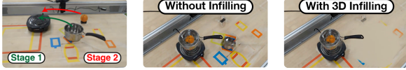
Figure 3: Scene-editing introduces artifacts, e.g., holes in the table (center) after moving the saucepan, which are removed via 3D Gaussian infilling (right).
